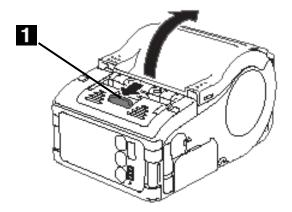
**Note:** If the red roller is not visible (lever cannot be pushed down), lift the edge (1) of the dispenser unit (2) slightly and slide it toward the front of the printer.
